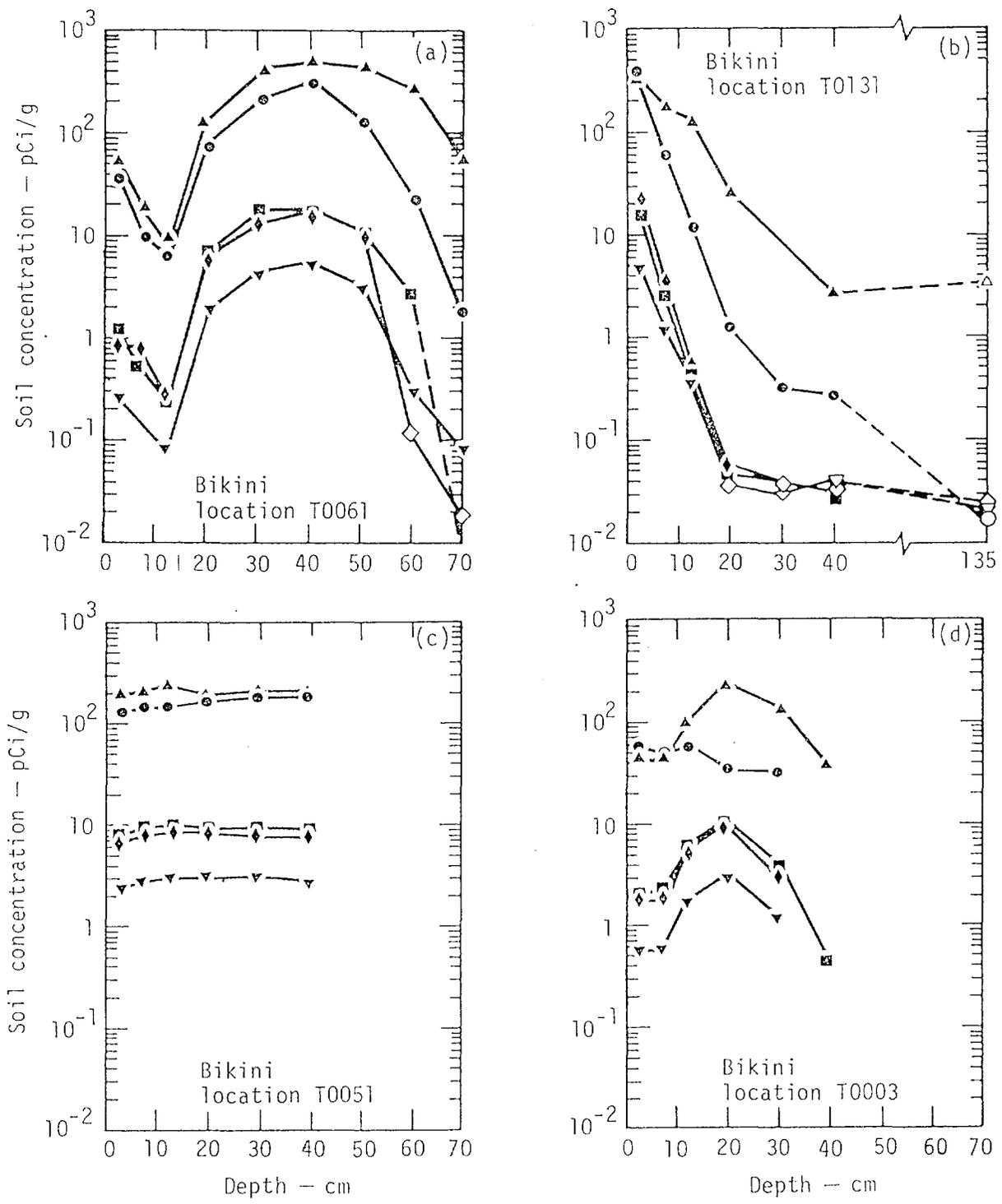
Fig. 4. Basic profile types from Gudiksen<sup>11</sup>: (a) erratic, (b) sharp drop-off, (c) uniform throughout, and (d) increasing then decreasing.
