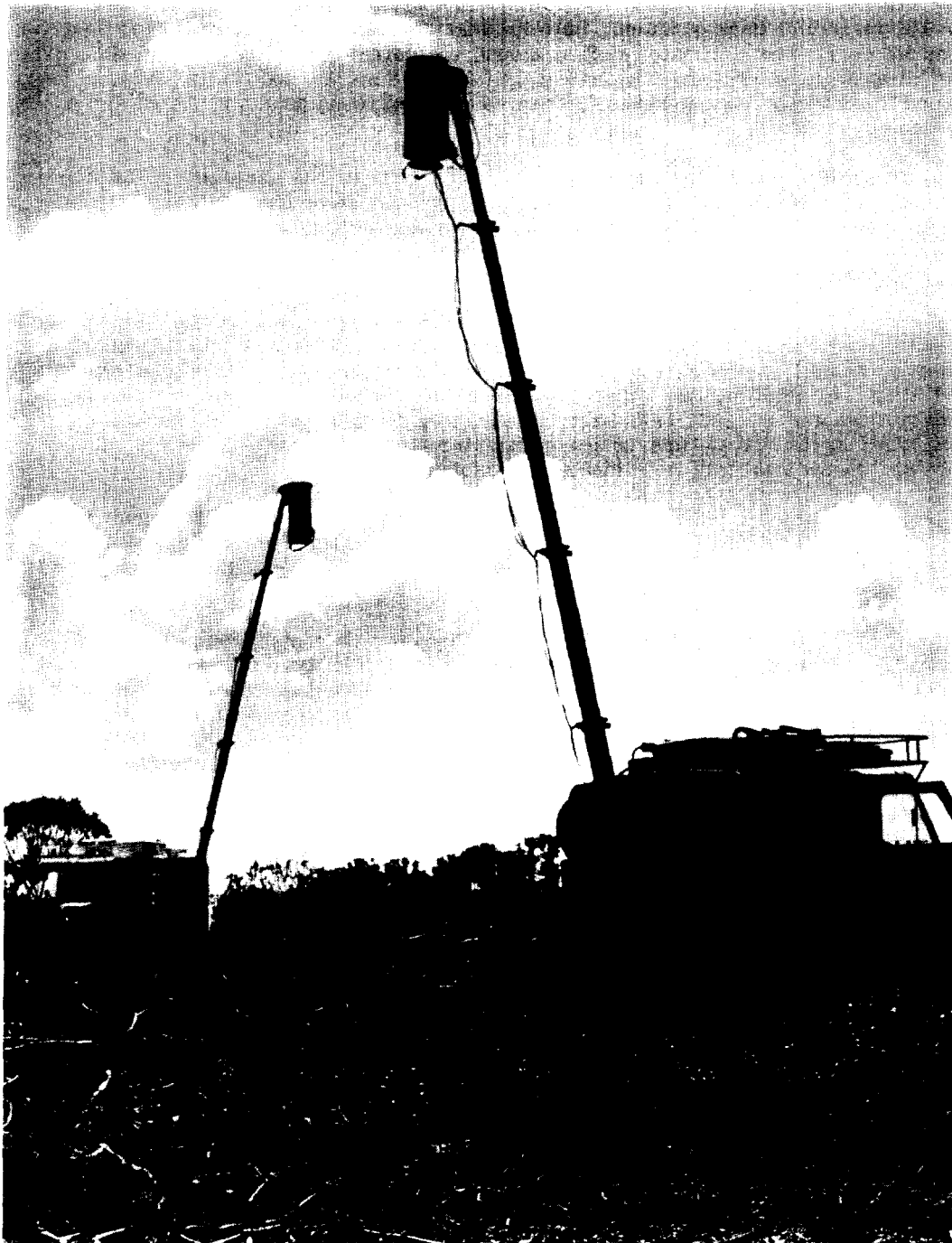
FIGURE 3-1. TWO IMPs SET UP IN A TYPICAL COUNTING MODE. The HPGe detector is housed inside the canister at the end of the retractable boom.
