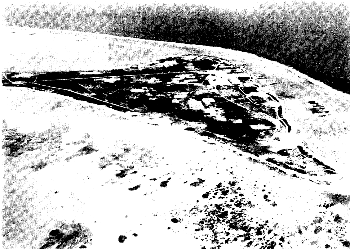
FIGURE 6-29. ISLAND JANET NEAR COMPLETION OF CLEANUP. The checkerboard pattern of light areas indicate locations of soil removal. A few months following the photo, vines had covered the clear areas so as to make them indistinguishable when seen from the air. Note the LLL research area toward the left point of the island. (February 1979)
